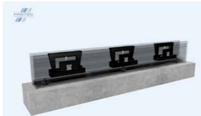
2. Slide retainers into position
